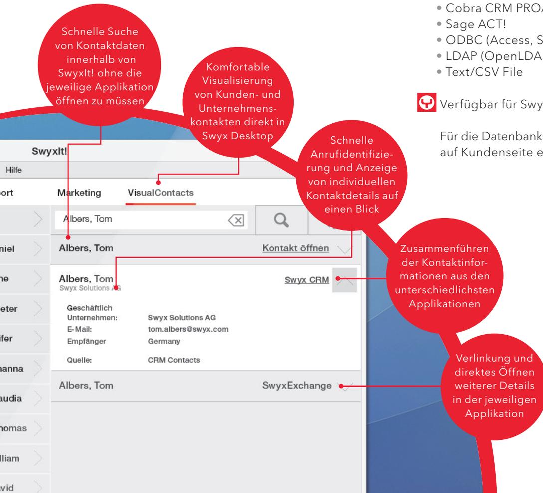
The screenshot shows the SwyxIt! VisualContacts interface. The main window displays a search for 'Albers, Tom' and a list of results. The first result is expanded, showing contact details for 'Albers, Tom' from 'Swyx Solutions AG'. The interface includes a search bar, a list of results, and a detailed view of a contact. Red callout boxes highlight key features:
